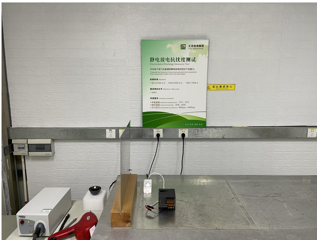
Test Setup Photo of Electrostatic Discharge Test
