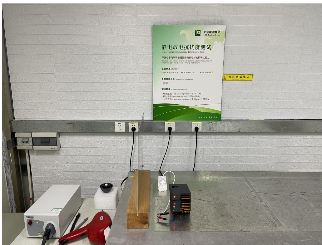
Test Setup Photo of Electrostatic Discharge Test
