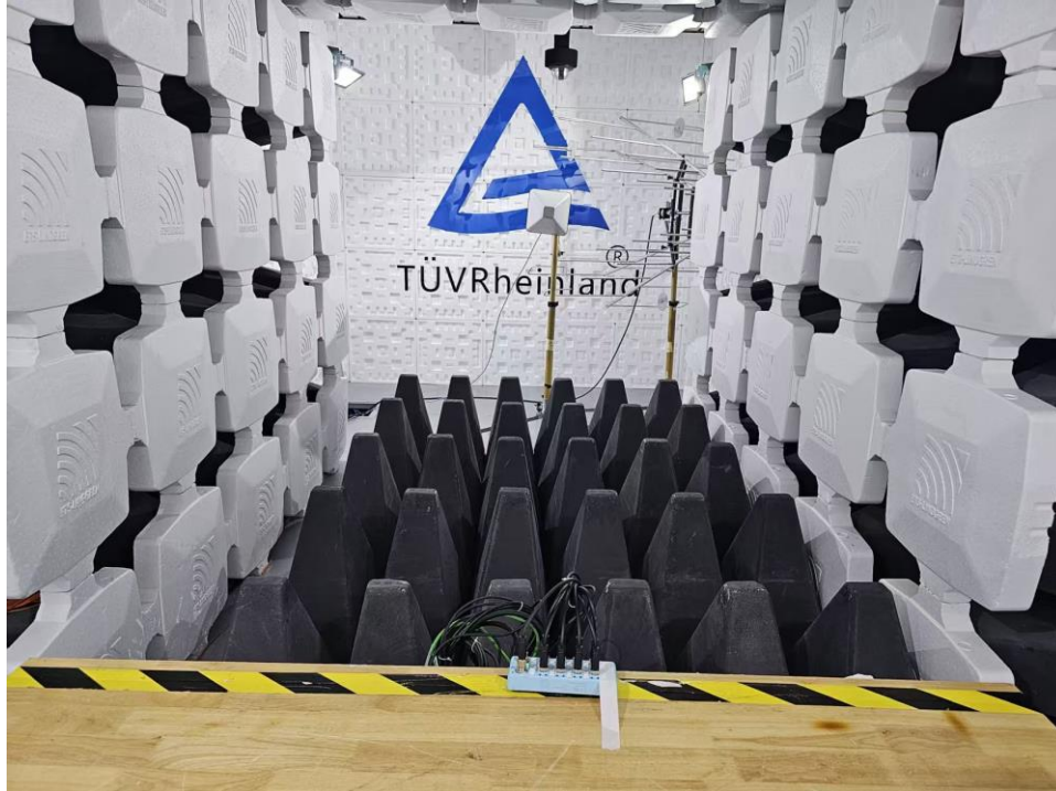
Photograph 4: Set-up for Electrostatic Discharges (ESD)
