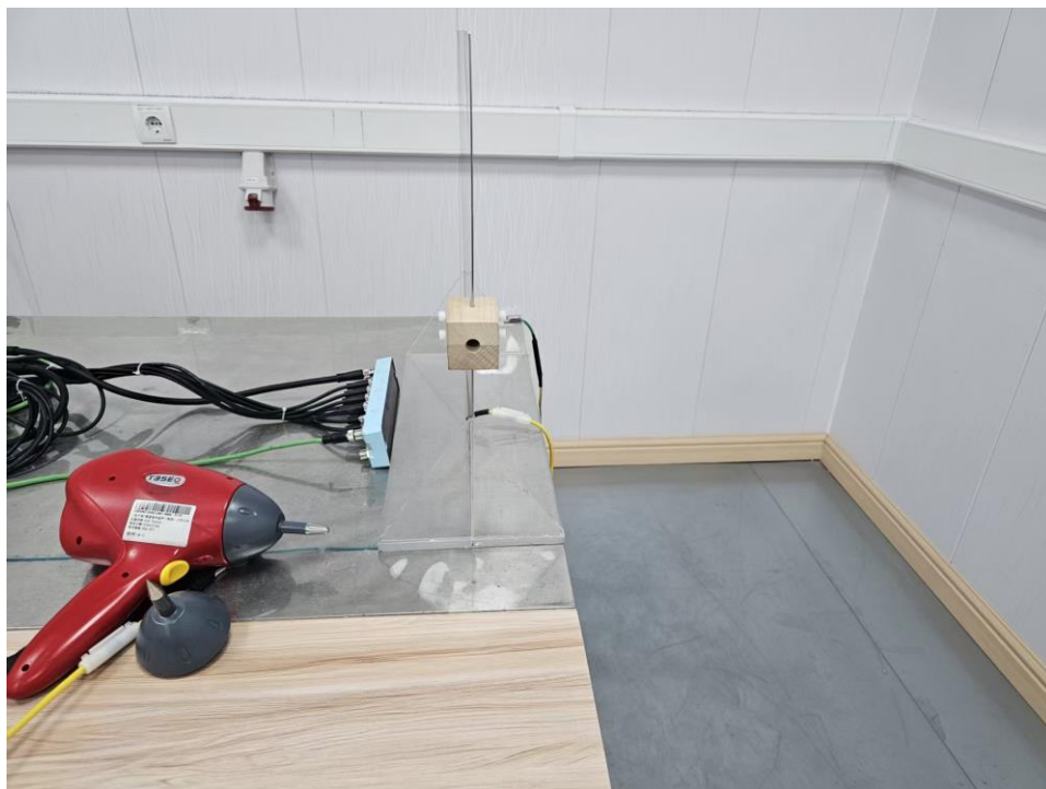
Photograph 4: Set-up for Electrostatic Discharges (ESD)
