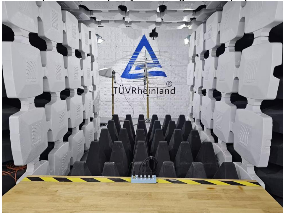
Photograph 2: Set-up for Radio-Frequency Electromagnetic Field (RS) Below 1GHz
