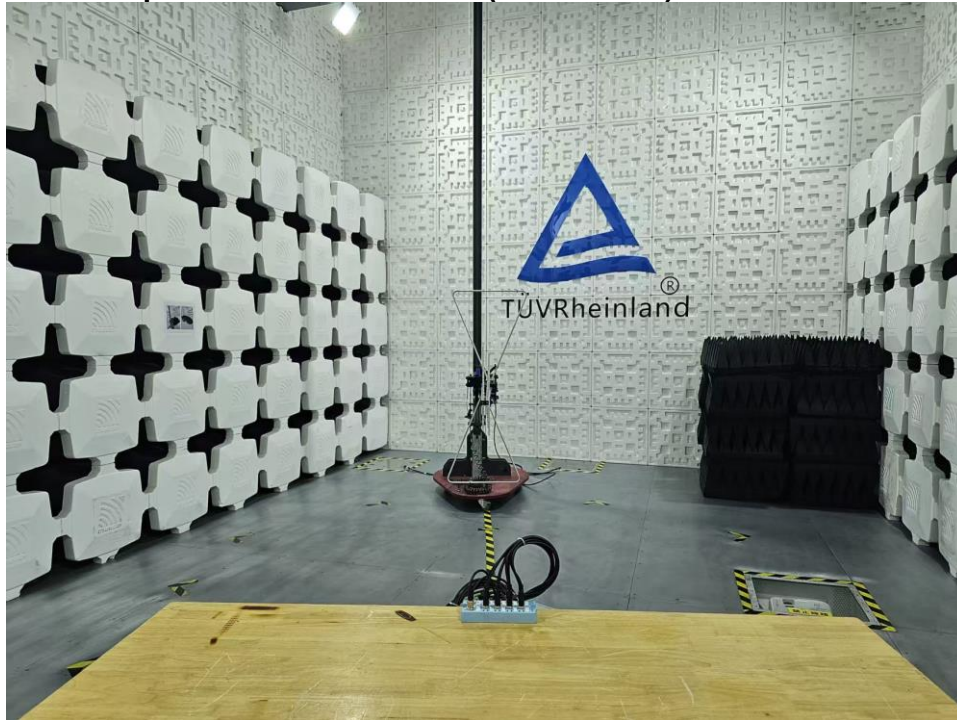
Photograph 1: Set-up for Radiated Emission (30-1000MHz)
