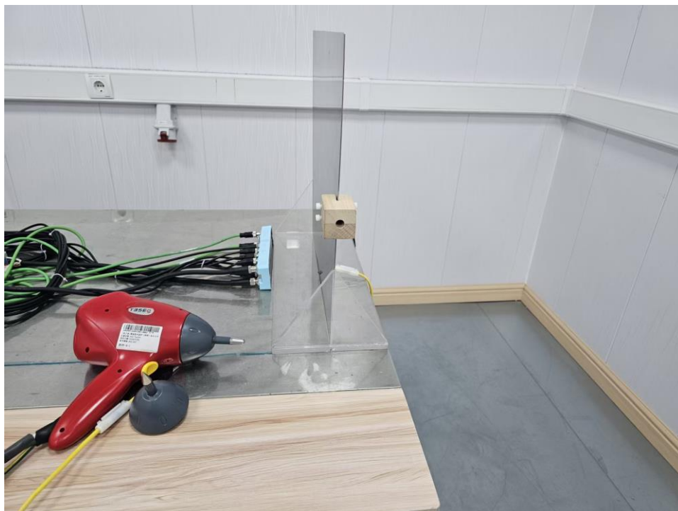
Photograph 4: Set-up for Electrostatic Discharges (ESD)
