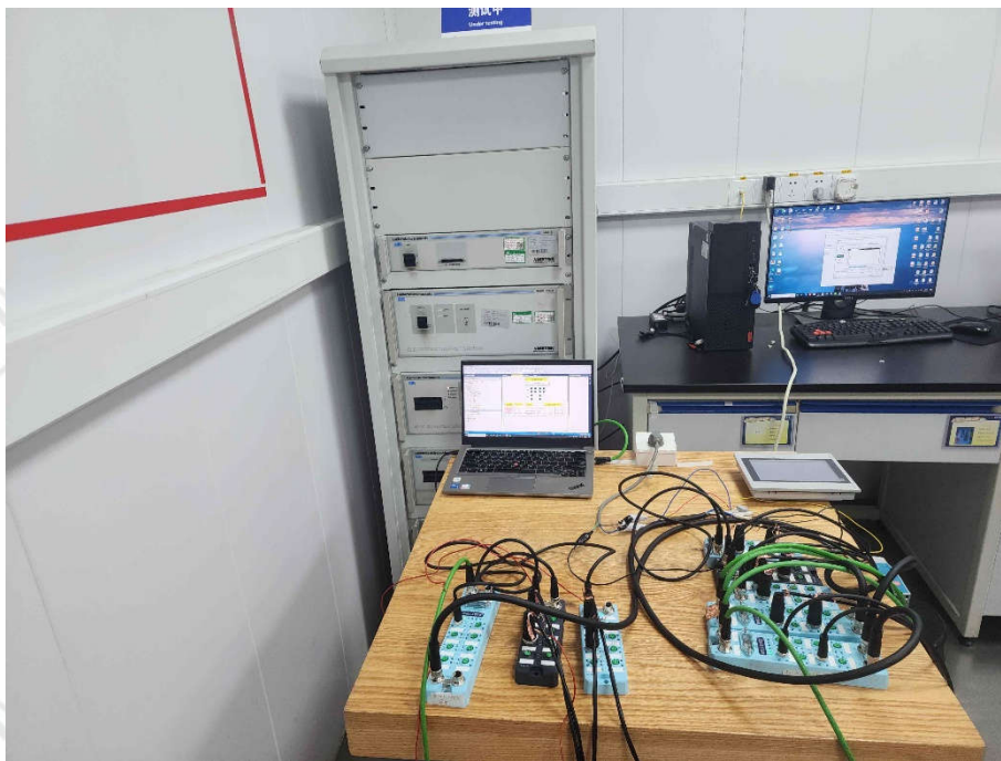
Voltage dips and interruptions Test Setup-1
