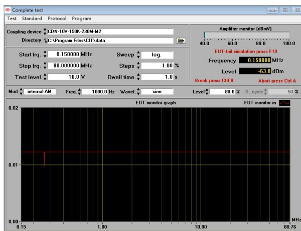
Figure2.3 Conducted Immunity Test (10V r.m.s)
